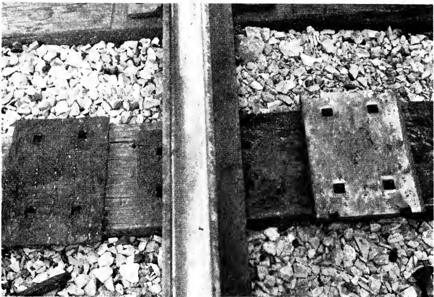
Fig. 13. Section 39. 11-in Bird 5-ply Duck-Burlap Tie Pad, Coated, After 58 months' Service in the Outer Rail of the North Spiral of the Long 4-1/2 th Curve.
